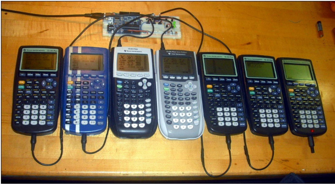
Fig. 1. A seven calculator setup; six of the calculators have been connected to the network.
