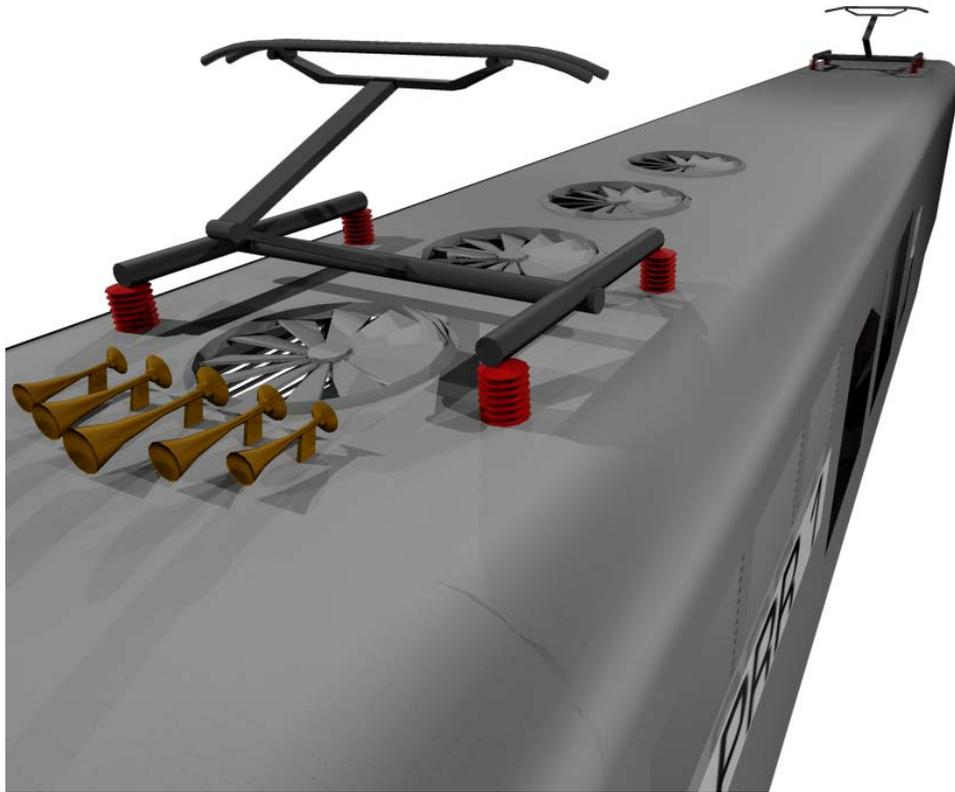
Fig. 15. Front top detail of horns, fans, pantograph.
