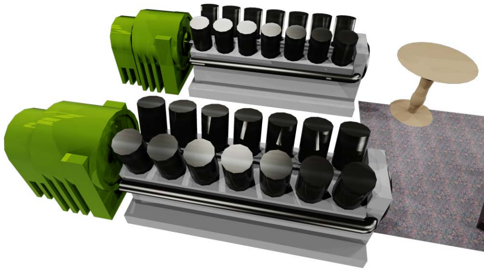
Fig. 6. From left to right, secondary alternators, main alternators, dual 14-cylinder engines, sitting room.
