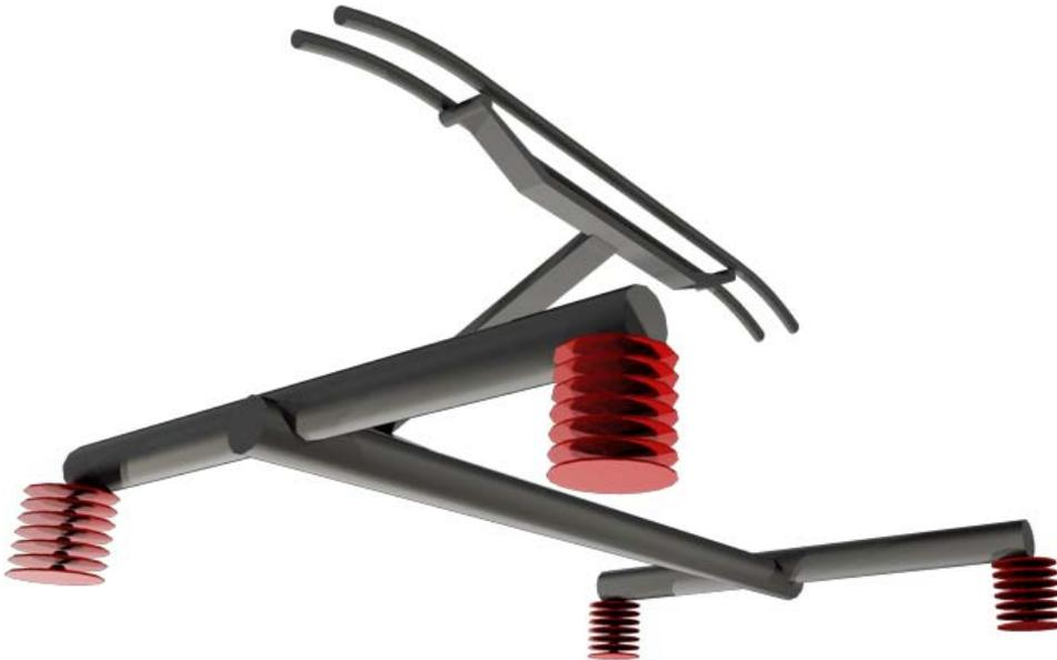
Fig. 13. Detail of rear pantograph assembly
