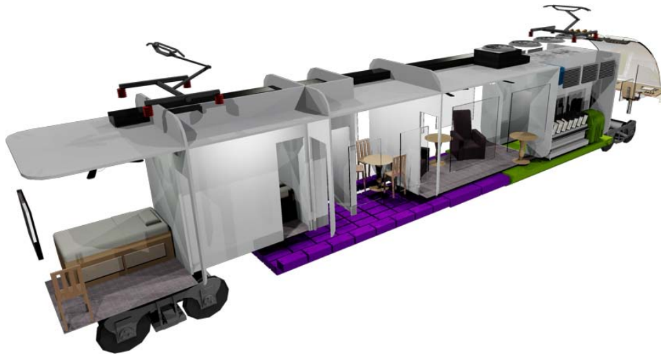
Fig. 4. Right-side view with outer body removed. Note battery/capacitor bank under floor.
