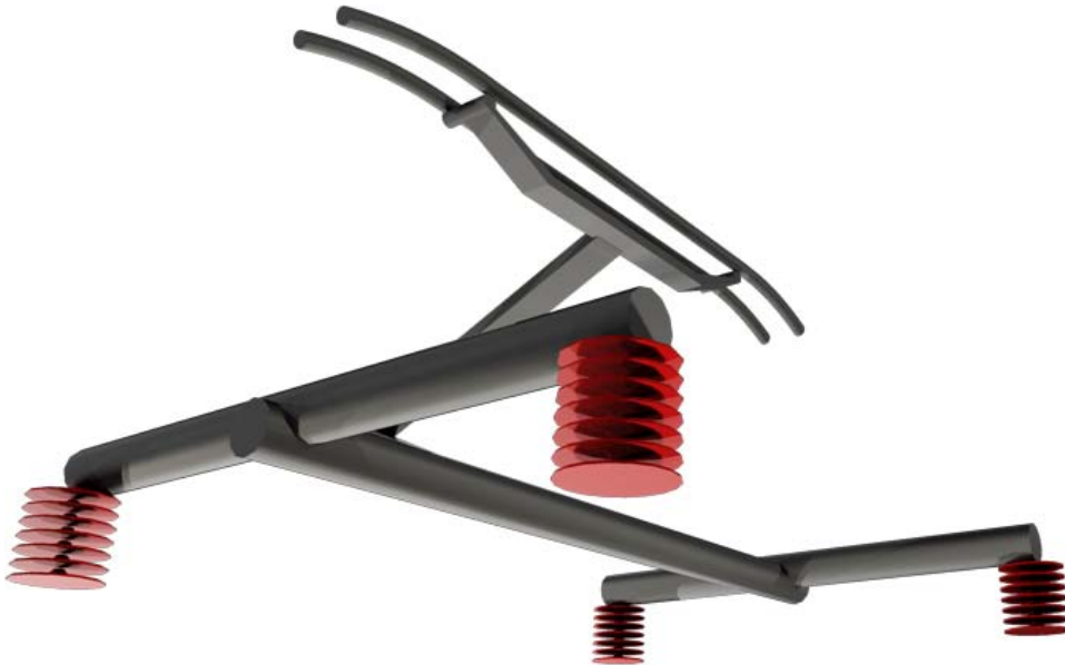
Fig. 13. Detail of rear pantograph assembly
