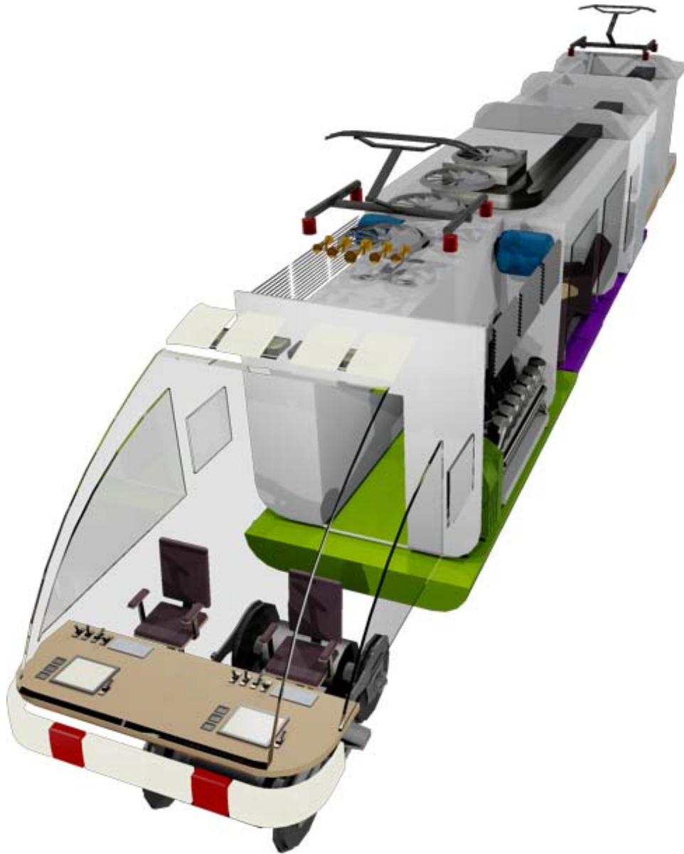
Fig. 3. Front-left view of CPRR1 with outer body removed. Note vent grates, engine, HVAC.
