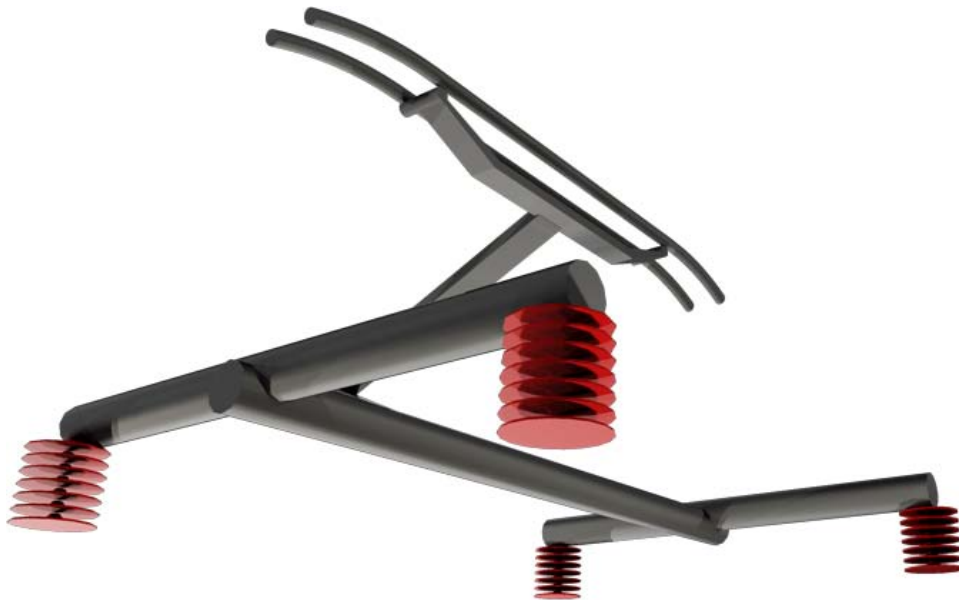
Fig. 13. Detail of rear pantograph assembly
